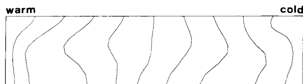
Figure 24. Isotherms at a depth equal to half the radius of the cylindrical crucible at Gr = 300,000
